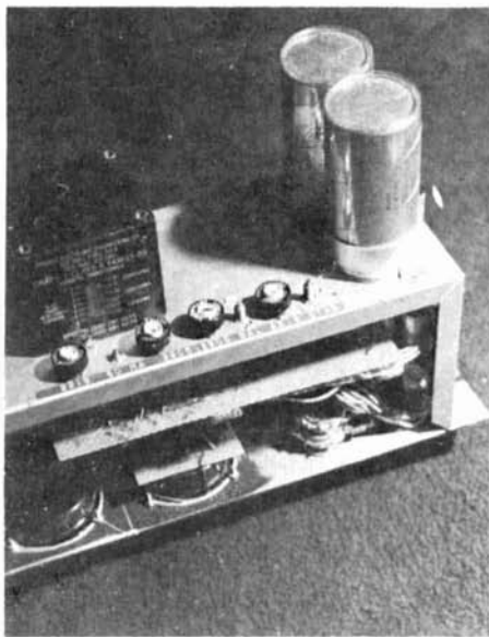
Rear view of the operational power supply showing the power transistors and adjusting controls.
